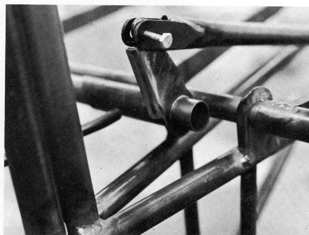
Left elevator horn attach fitting.
