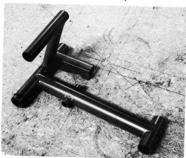
Rudder and brake pedal assembly.
