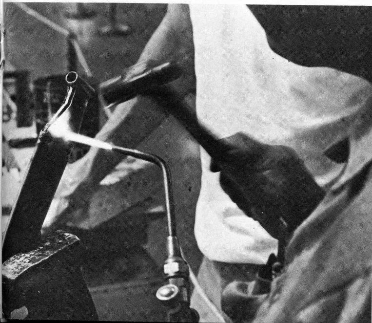
Welding center section end struts.
