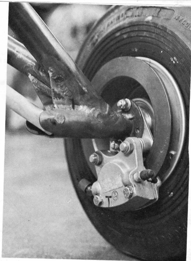
Landing gear axle and brake assembly. 5:00 x 5 wheels are shown. Reinforcing straps on axle at shock strut attach have yet to be welded on.
