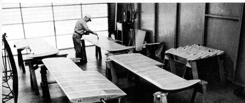
The wing panels and ailerons receive their final coat of clear dope prior to being sprayed silver. Note that all wing ribs and edges are covered with pinked tape.
