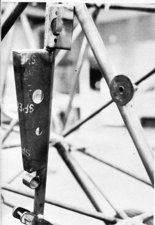
Ignition and mixture control bracket.
