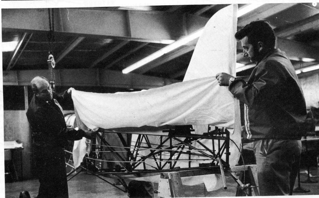
Aligning fabric for fuselage cover, a dope primer should be sprayed on all metal surfaces before covering.
